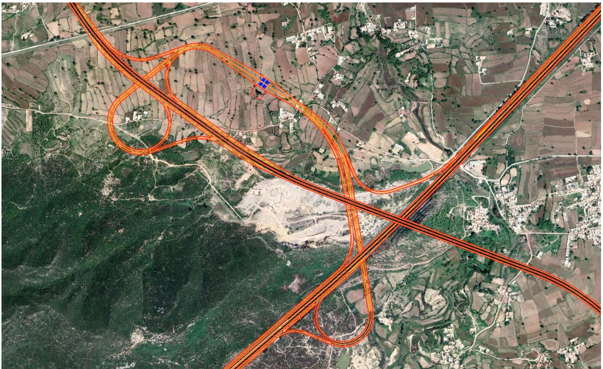
Double Trumpet Interchange at Murat (M-2) crossing
