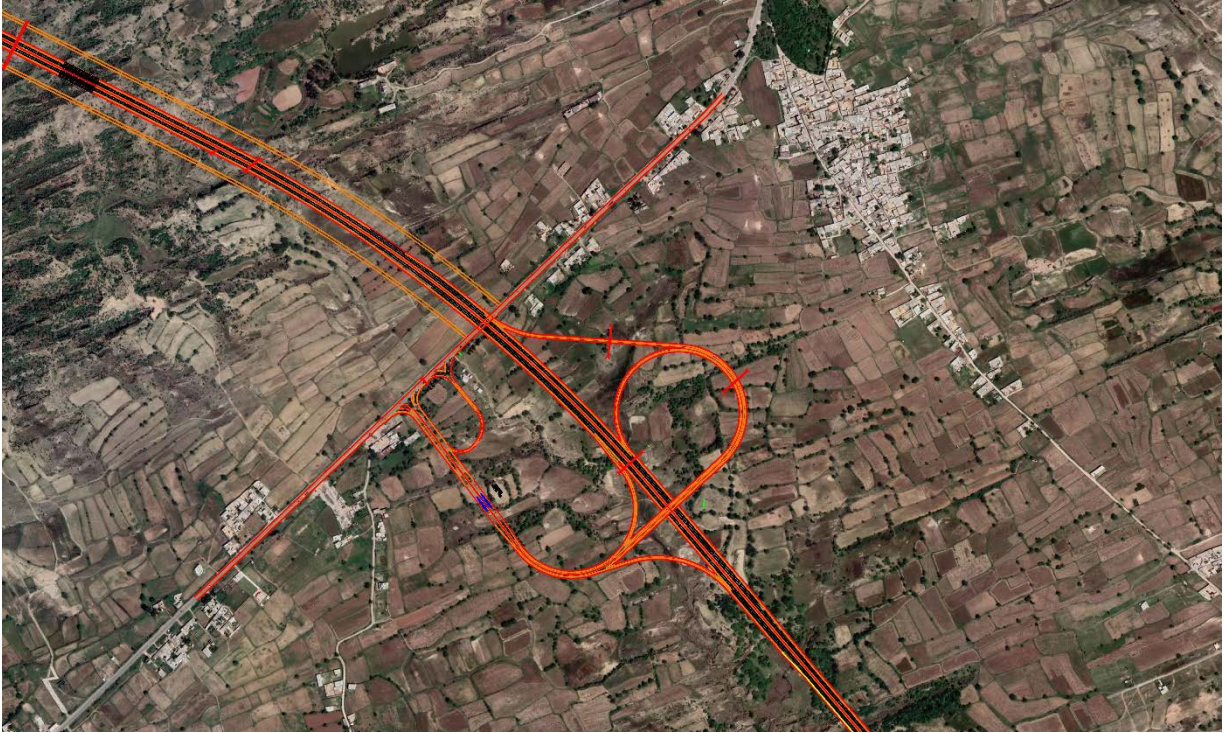
Partial Clover leaf interchange Chakri Road crossing (Future)
